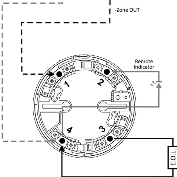
**NOTE:** Positive terminal of remote indicator should be connected to terminal 4.
