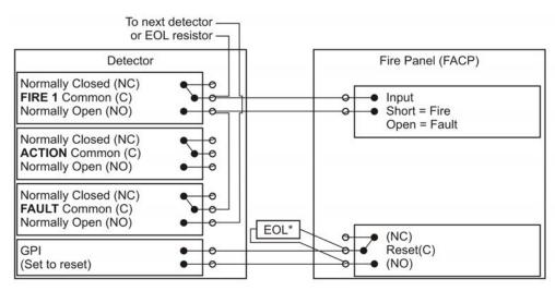
Figure 2-13: Typical wiring to a fire panel with EOL
