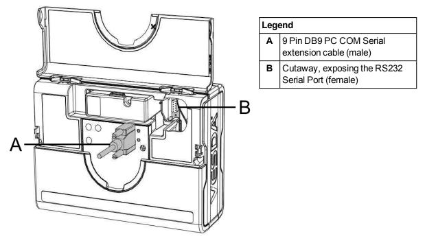
Figure 2-15: 9 pin connector and RS232 serial port
