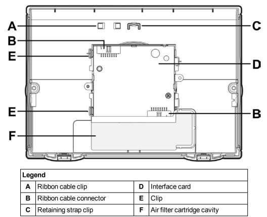
Figure 2-6: Inside view of the front cover (as it would appear inverted)
