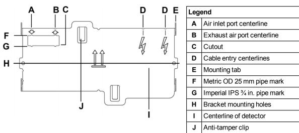
Figure 2-4: Mounting bracket orientation for upright and inverted mounting
