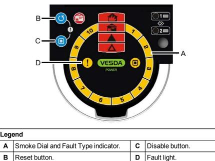
Figure 6-5: Smoke level and fault condition display
