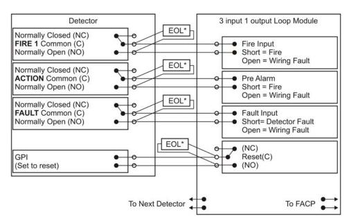
Figure 2-14: Addressable Loop Module with EOL
