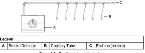
Figure 3-2: Capillary tubes, single pipe
