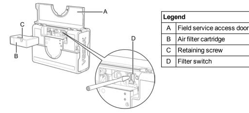
Figure 9-2: Filter replacement
