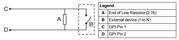
Figure 2-10: Triggering of GPI
