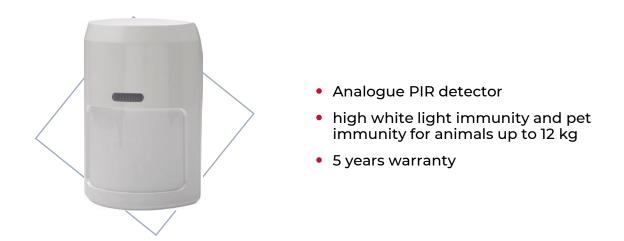
TITAN AG is an analogue PIR detector suitable for use in residential, commercial and office buildings. TITAN AG has high white light immunity and pet immunity for animals up to 12 kg. The detector is also equipped with adaptive temperature compensation. TITAN series detectors have a 5year warranty.
