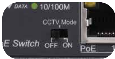
CCTV Mode Switch
