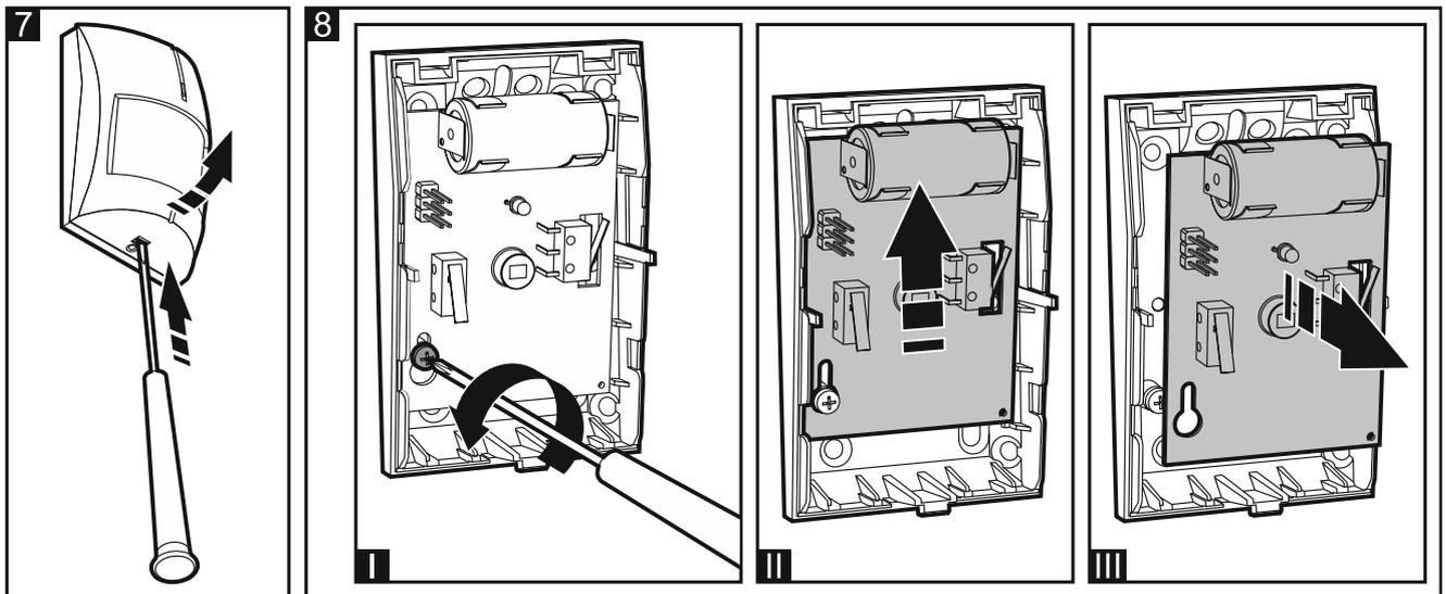
3. Install the battery in the detector.
