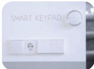
Rotate the Keypad to Arm the system for checking the connection with the Hub.
