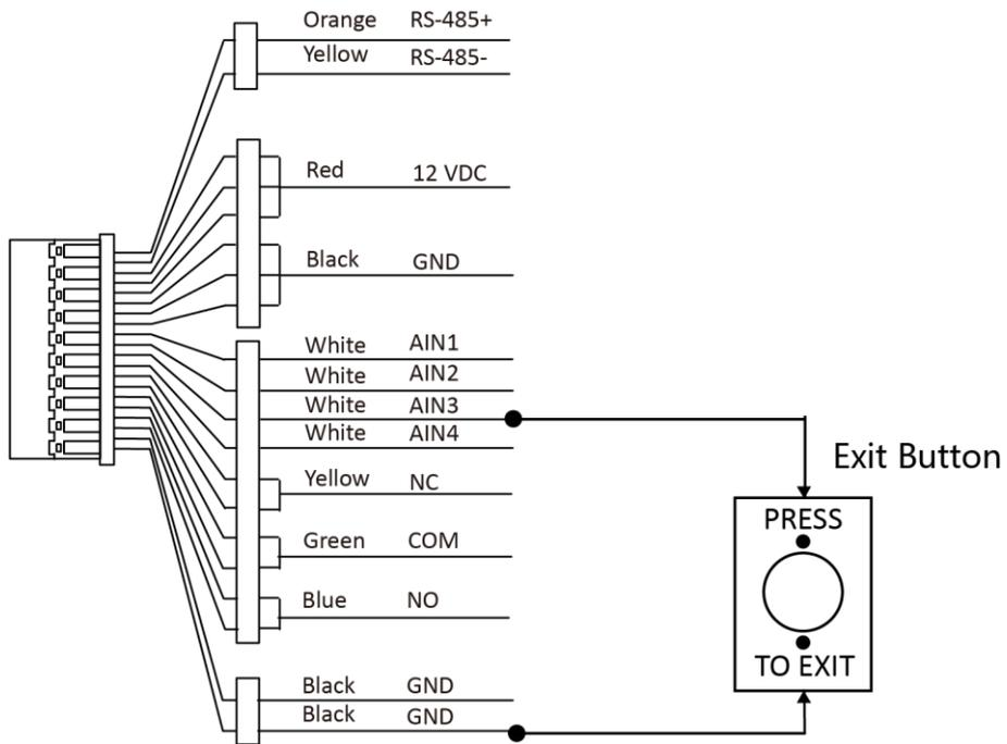
Figure 2-4 Exit Button Wiring
