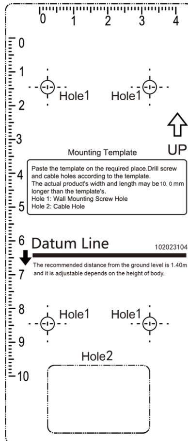
Figure 3-2 Mounting Template
