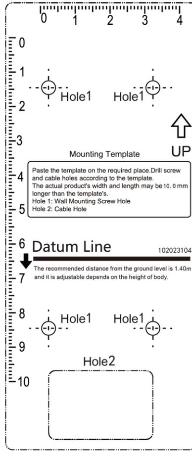
**Figure 3-4 Mounting Template**
