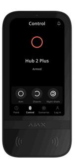
KeyPad TouchScreen can arm and disarm the entire facility or specific groups, and activate **Night Mode**. Use the **Control** • tab to change the security mode. You can control the security using KeyPad TouchScreen through:
