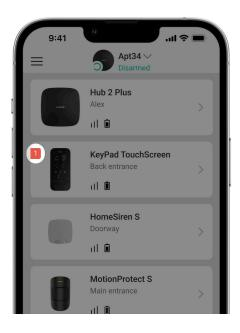
When a KeyPad TouchScreen malfunction is detected, the Ajax app displays a malfunction counter on the device icon. All malfunctions are indicated in the keypad's states. Fields with malfunctions will be highlighted in red.
