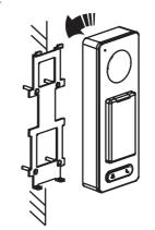
5.Push the terminal in the mounting plate from bottom up.
