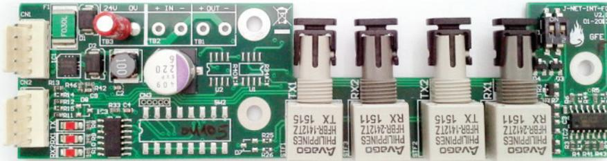
The J-NET-INT-FO interface modules allow GFE's range of panels to be interfaced to repeaters and/or sub-panels using Fibre Optic cable using a common data communication loop in a ring topology. These units also use a doubled redundant data communication loop for extra security and reliability.
