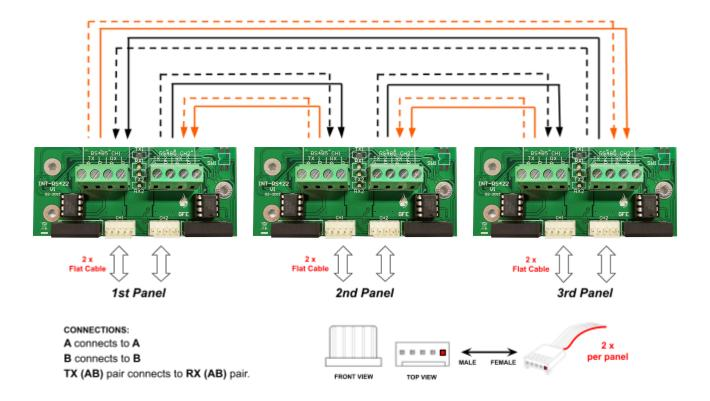
The following image shows a single wiring connection, normally used for CHAMELEON Display extension or BMS connection.
