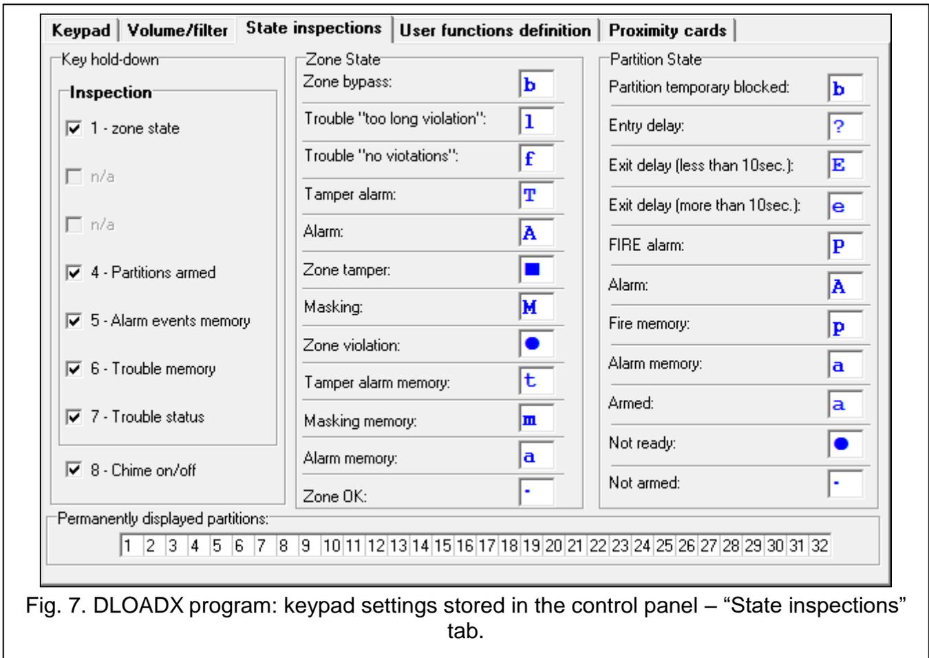
Fig. 7. DLOADX program: keypad settings stored in the control panel – “State inspections” tab.
