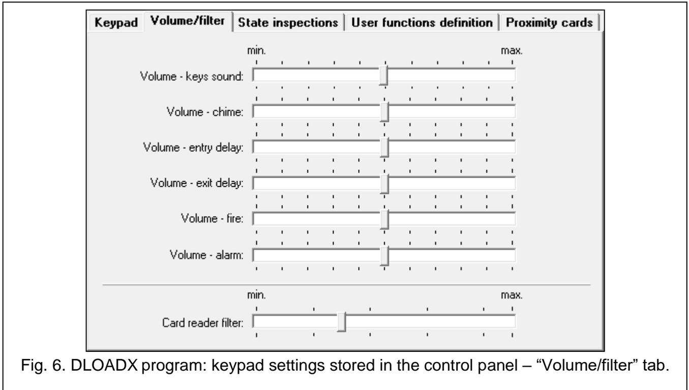
Fig. 6. DLOADX program: keypad settings stored in the control panel – “Volume/filter” tab.
