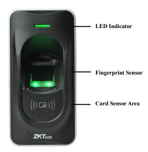
❖ LED indicator: The LED indicator is used to display reader operation results and exceptional statuses which are defined as follows: **Operation succeeds:** The green indicator is solid on for one second, at the same time the speaker play one long beep.
