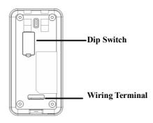
**Dip Switch:** 1-4 switches are used to set the RS485 communication address (device ID). Number 5 switch is idle. And the number 6 switch is used to set the terminal
