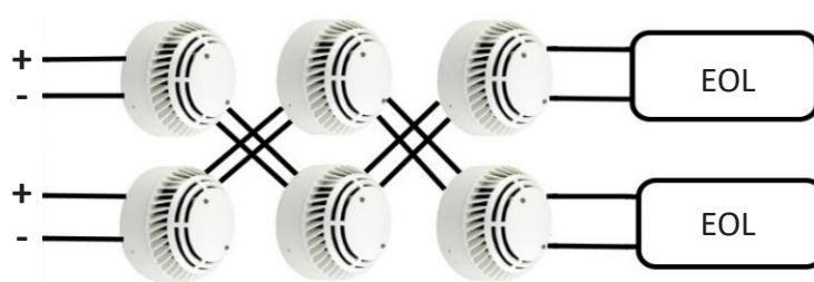
Figure 10: Z1 and Z2 with interlaced connection and capacitive end-of-line CAP 50V 10 \mu F
