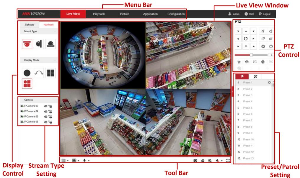
Figure 4-2 Live View Page (Hardware Decoding)
