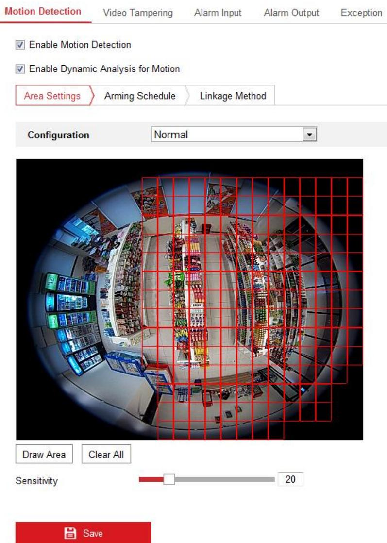
Figure 5-44 Motion Detection Settings
