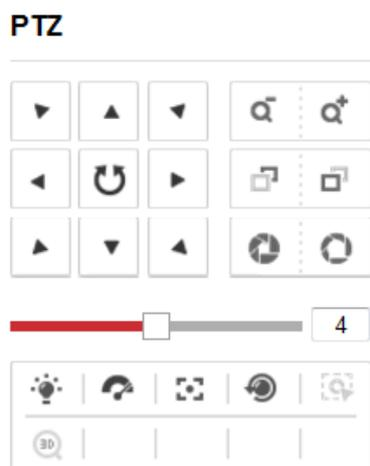
Figure 4-6 PTZ Control Panel
