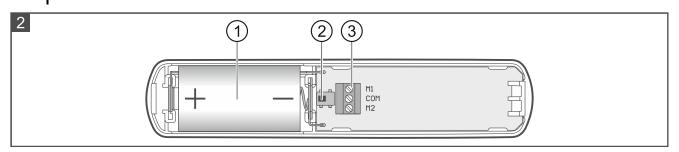
Fig. 2 shows the detector inside after opening the enclosure.
