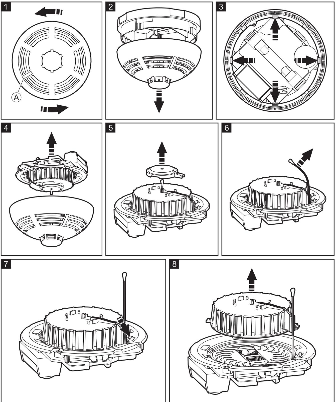
8. Using a soft brush or compressed air, clean the labyrinth in the cover and the base of the optical chamber, paying attention to the recesses where the LEDs are installed.
