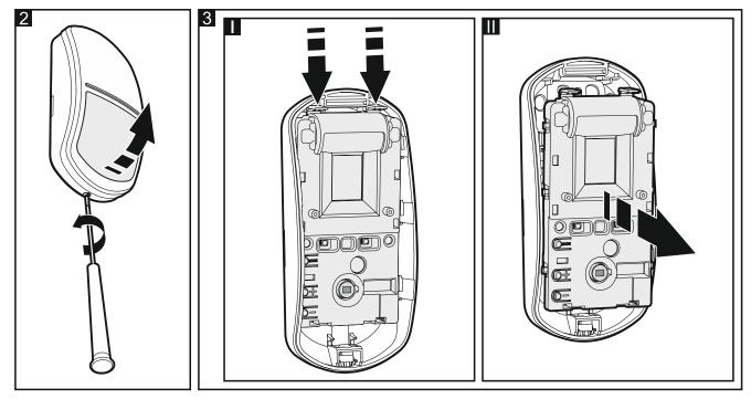
3. Install the battery and add the detector to the wireless system (see the ABAX 2 / ABAX controller manual or the INTEGRA 128-WRL control panel installer manual). The sticker with serial number which shall be entered when registering the detector in the system can be found on the electronics module.
