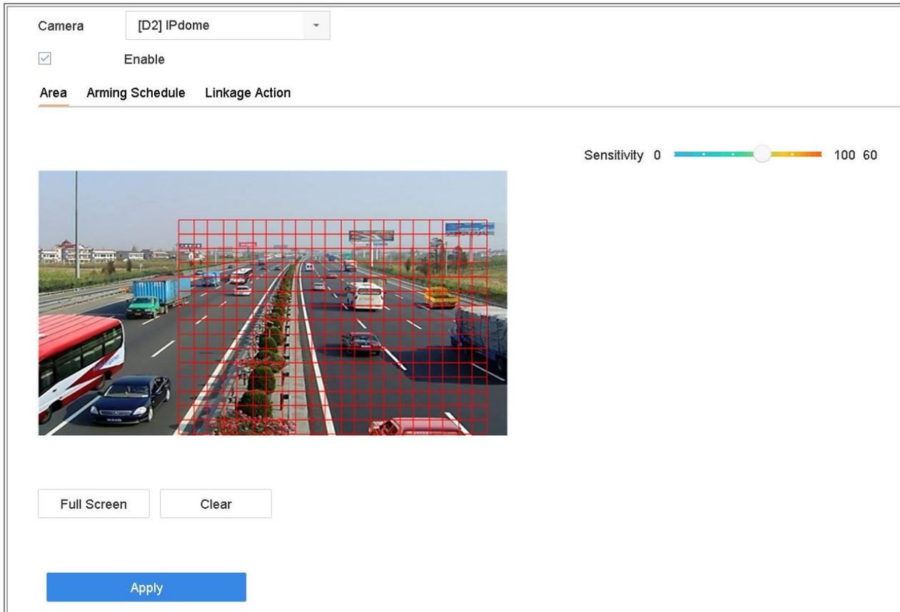
Figure 11-5 Set Motion Detection
