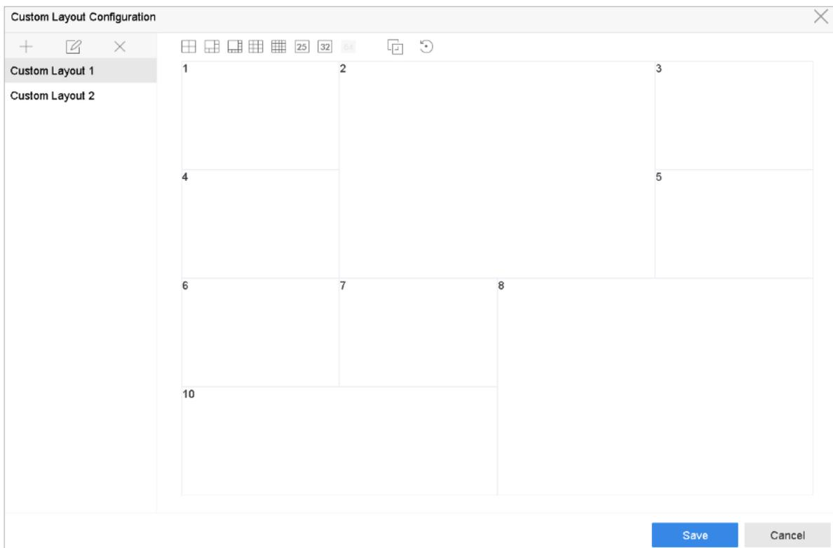
Figure 5-4 Configure Live View Layout
