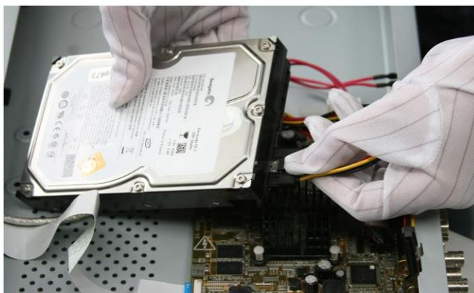
Figure 2-3 Connect Power Cable
