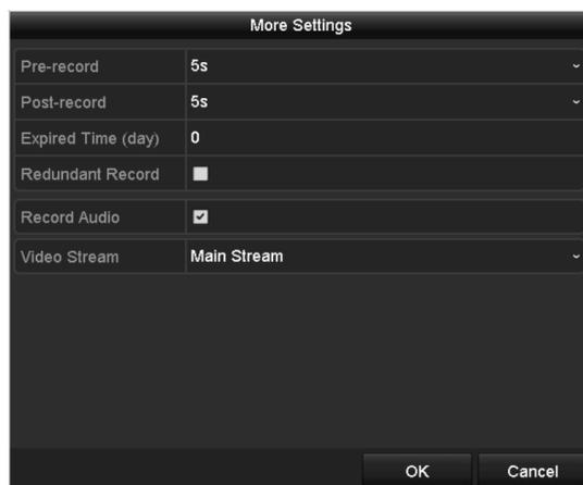
Figure 5. 3 Recording Parameters-More Settings
