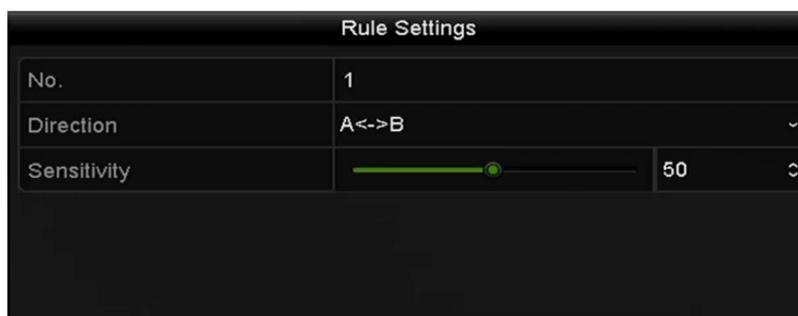
Figure 8. 13 Set Line Crossing Detection Rules
