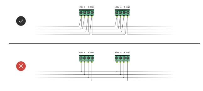
+24V — power A, B — signal terminals GND — ground
