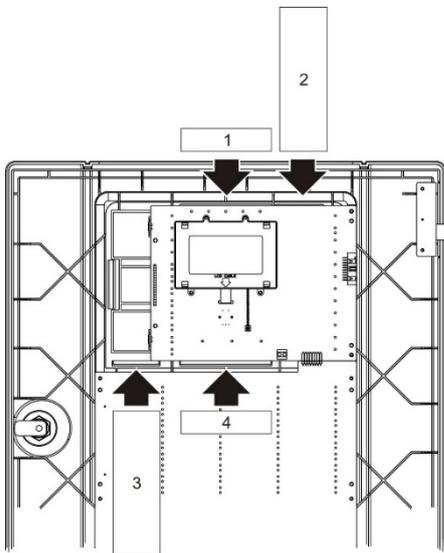
The inserts are numbered 1, 2, 3, and 4, and are inserted at the location indicated (with the printed area facing the front of the control panel).
