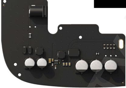
12V PSU for Hub 2 is a power supply unit, connecting the Hub 2 control panels to 12 volt DC sources. This is an electronic board, replacing the standard 110/230 V power supply unit in the body of the device.
